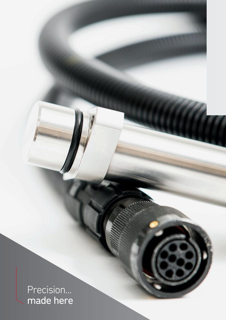
4 Channel Speed Sensors are made to operate in harsh environments by sensing a ferromagnetic target wheel, or module gear. Hall Effect technology is used to detect a change in the magnetic field when a target or gear wheel is rotated in front of the Speed Sensor.
